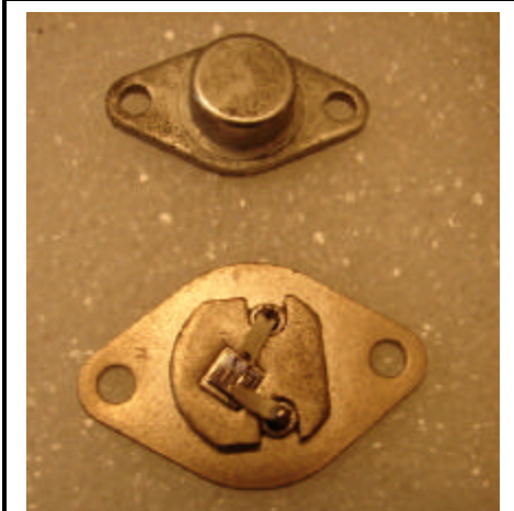
TOP: A TA 2700, 1965 transistor prototype (note lack of markings). The transistor was mainly used for high voltage Class A audio output stages and line operated equipment such as radios and phonographs. Its thermal resistance was improved by use of an internal, copper heat sink. A new 2-lead (stiff) stem was used in place of the 3-lead (flexible) stem used on the TA 2301.
