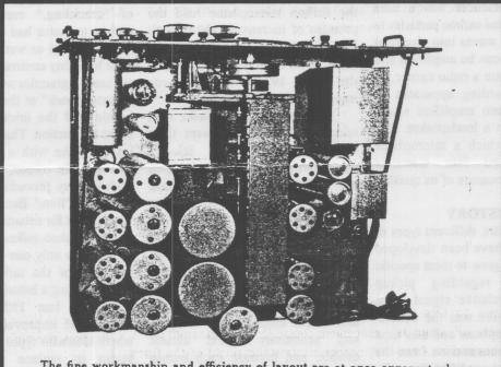
The fine workmanship and efficiency of layout are at once apparent when examining the chassis of the AR-60. Note the 8-gang tuning condenser.
