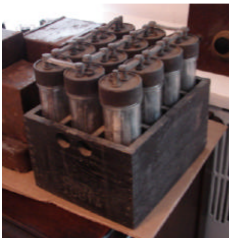
Willard wet cell "B" (24 volt) battery
