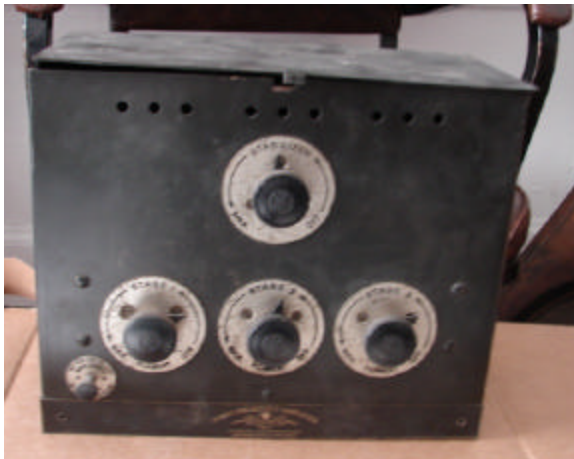
Radiola III (WD-11 has open filament)
