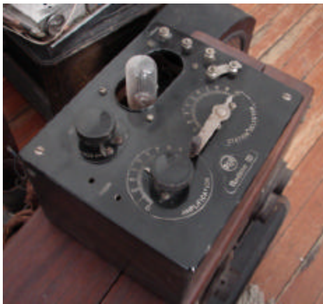
Radiola III (WD-11 has open filament)
