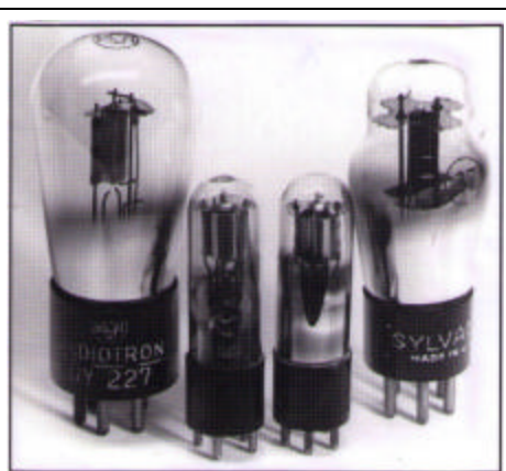
Miniature "27's" used in the Radio Products clock radio in comparison to their standard big brothers.
