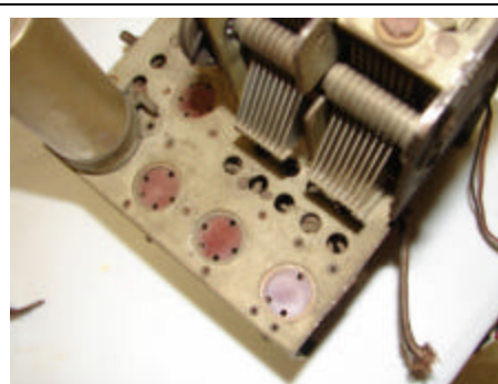
Tube sockets that hold the miniature type "27" tubes.
