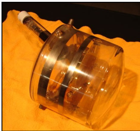
Examples of a Farnsworth image dissector and Zworykin Iconoscope provided by Mike.
