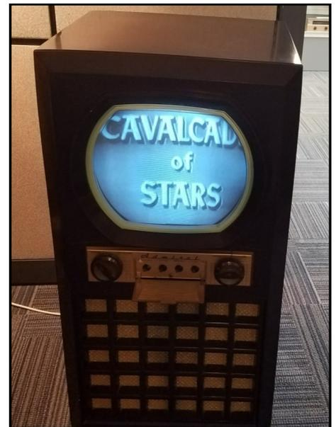
**This 1949 Admiral Model 22X12 is identified by its rectangular grill pattern and round picture tube. Later models employed rectangular 14-inch, 16-inch and 17-inch tubes.**
