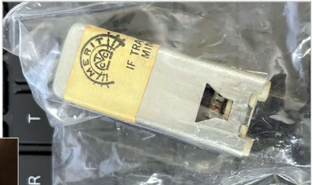
Example of IF transformer with ceramic capacitors inside
