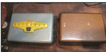
The Motorola 708 (left) used in 1941-1947 Plymouths, Chryslers, Dodges and DeSotos. The Tucker radio is similar but uses a different head and has a hammertone, copper finish.
