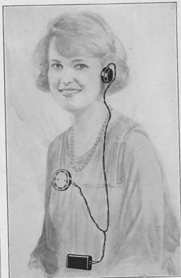
Outline Sketch of Photograph on Page 3, Showing Correct Position of Every Part of the Hidden Acousticon
