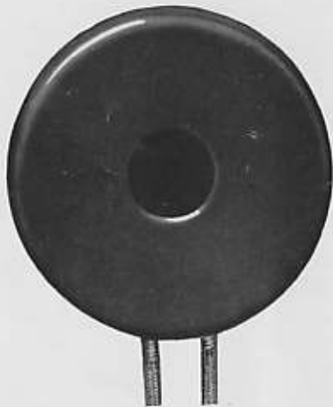
Earpiece, Front View, Showing Orifice to be Placed Over Opening Into the Ear
