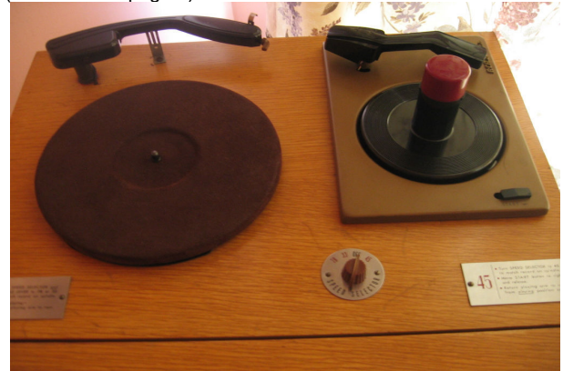
The 15E uses 2 turntables to play all record speeds
