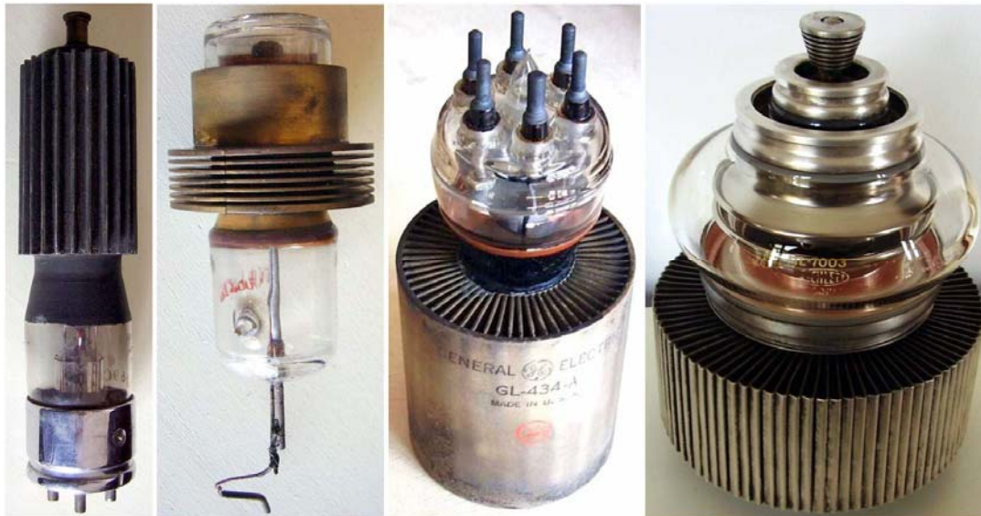
Fig. 17 - Power tubes with air-cooled external anode made of copper sealed to the glass bulb. Radiating fins are brazed to the copper surface.
