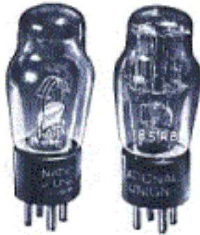
Fig. A. The type 1A1 Current Regulator type of glass-envelope ballast tube is for use in operating 2-V tubes from a 3-V "A" supply. The type 185R8 Line Ballast tube replaces the resistor cord in AC-DC sets; it is also provided with a tap for two 6-8 V pilot lights.
